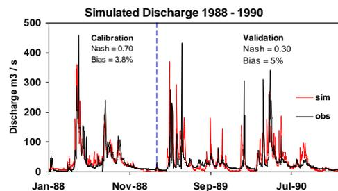
**Fig. 6** Observed and simulated discharge
