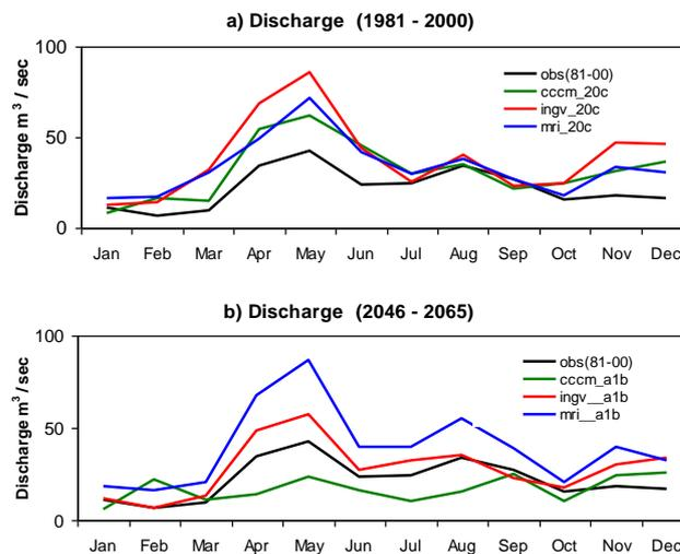
**Fig. 7** Mean monthly discharge using GCM corrected rainfall for 1981-2000 (a) and 2046 -2065 (b).
